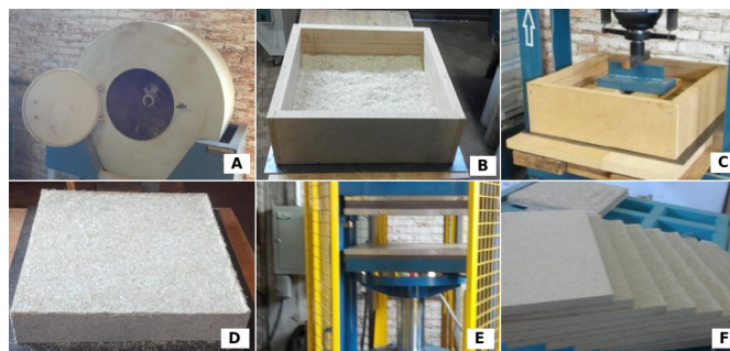
Figure 2. Panel manufacture: (A) Warp slasher; (B) Mattress forming; (C) Manual hydraulic press; (D) Particle Mattress; (E) Motorized hydraulic press; (F) Finished particleboards.
