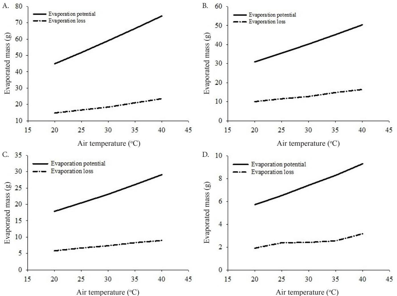
**Figure 3.** Evaporation potential of water inside the climate chamber and water loss by evaporation, which was determined based on the air enthalpy, as a function of temperature and distinct values of relative humidity. A. 30%; B. 50%; C. 70%; and D. 90%.
