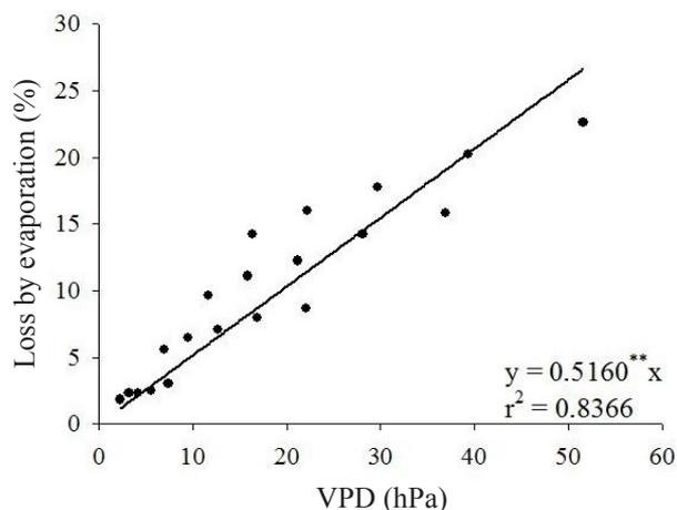
**Figure 4.** Relation between liquid percentage loss due to evaporation and vapor pressure deficit (VPD) by spraying using the spray nozzle LD11002 at the working pressure of 300 kPa.
