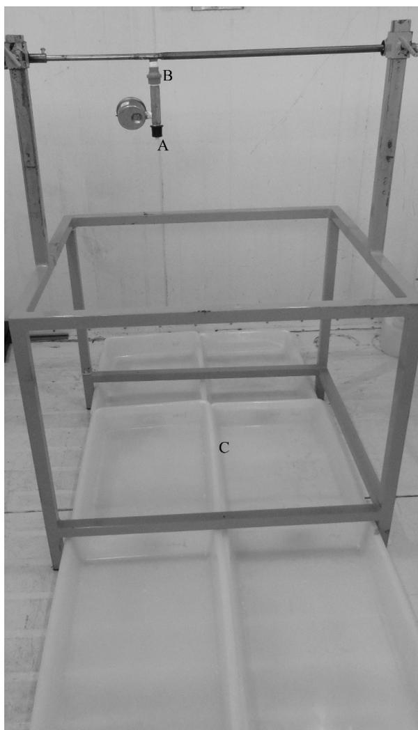
**Figure 1.** Experimental system built to estimate sprayed liquid loss by evaporation as function of the air psychrometric conditions. (A) spray nozzle; (B) constant pressure valve; (C) trays.
